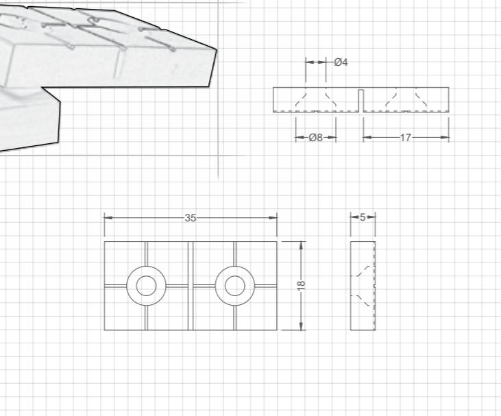
Front View: 35 mm width, 18 mm height, 5 mm thickness.
